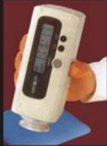
Minolta Colour Matching Reader Check the colour difference between two samples, with running production and development of new colour
